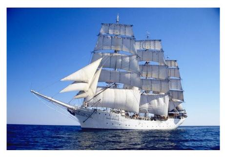
Christian Radich is a class A Tall Ship built in Norway in 1937. A regular visitor to Lerwick, the ship's home port is Oslo. Christian Radich is a white, steel hulled ship measuring 62 metres in length, with a total length of 73 metres including the bowsprit, it can carry 85 trainees and 30 permanent crew.
