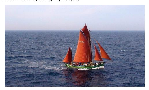
Shetland's very own Tall Ship - Swan - is a Class B, Gaff Ketch. The vessel was launched in 1900 in Lerwick, originally built as a Fifie herring drifter. Swan has a 20.4 metre long, green wooden hull, the total length being 26.10 metres. Swan's homeport is Lerwick, Shetland and the vessel can carry 10 trainees and 5 crew.
